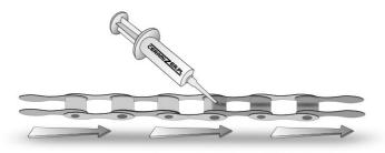
Apply the lube evenly on the mid part of the link. During first chain turns it will be distributed all over the whole surface. The consistency of the lube enables it to penetrate under the chain seals and thus reach all working areas of chain and sprockets. Do not apply excessive quantities of lube on particular links.
